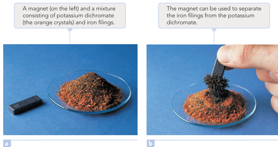
Figure 1-5 Physical separation of the two components of a mixture using the magnetic properties of one of the mixture components.
